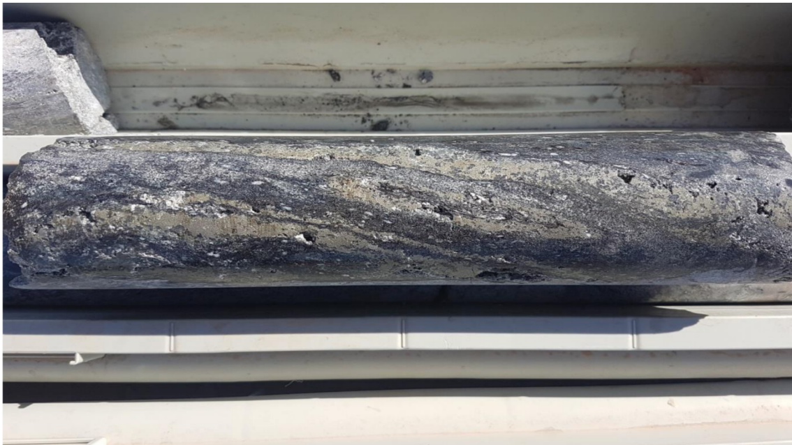
[Figure 5] Mount Skipper Project: MSD 19-01 core showing folded, semi-massive bands of pyrite ± pyrrhotite rare chalcopyrite host in coarse spotted cordierite and sillimanite rock types.
