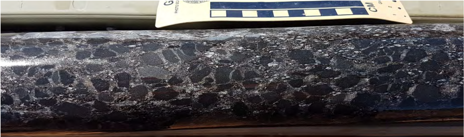
Biotite-sillimanite-quartz schist with strong muscovite retrograding and unusual coarse, angular, grey porphyroblasts retrograded to fine muscovite . Porphyroblasts may be after cordiorite but now mostly very fine-muscovite (needs petrology).
