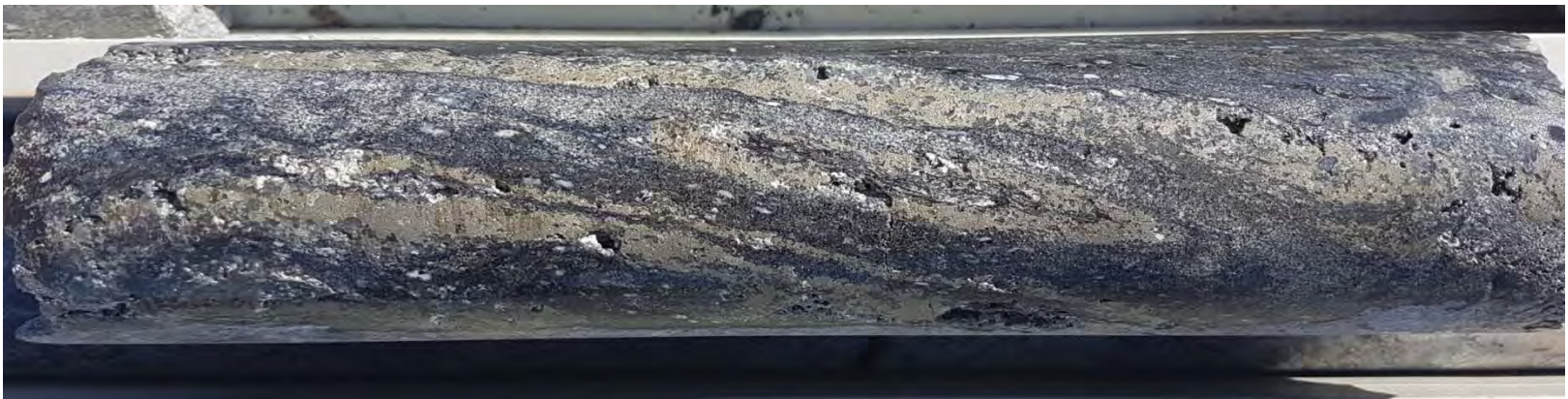
Semi-massive pyrite veins and bands with trace chalcopyrite and pyrrhotite. Pyrite bands appears to be folded.
