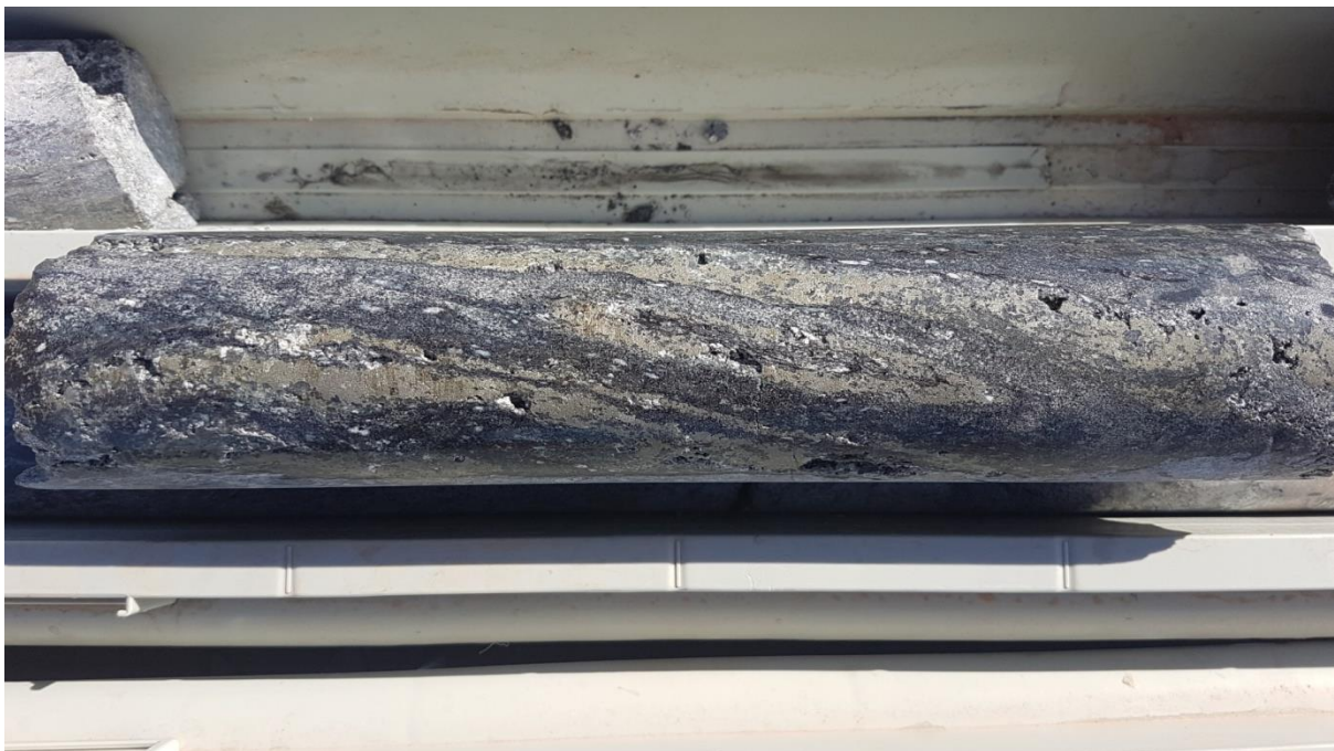
[Figure 2] Mount Skipper Project: MSD19001 core showing folded, semi-massive bands of pyrite with minor weakly magnetic pyrrhotite and rare chalcopyrite host in coarse spotted cordierite and sillimanite-quartz rock types.
