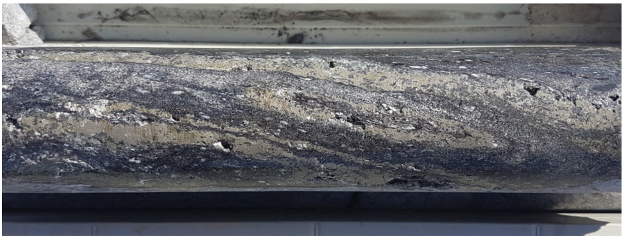
[Figure 5] Mount Skipper Project: MSD 19-01 core showing folded, semi-massive bands of pyrite ± pyrrhotite rare chalcopyrite host in coarse spotted cordierite and sillimanite rock types.
