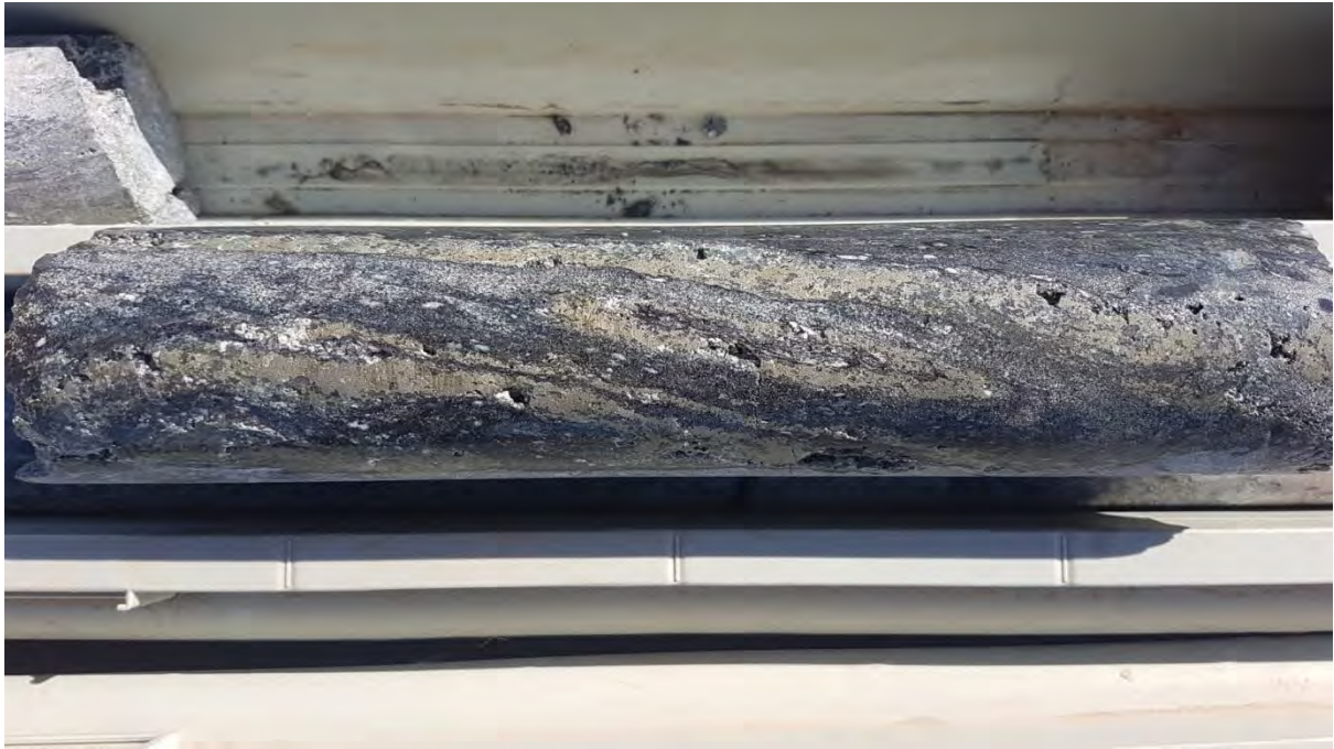
[Figure 2] Mount Skipper Project: MSD19001 core showing folded, semi-massive bands of pyrite with minor weakly magnetic pyrrhotite and rare chalcopyrite host in coarse spotted cordierite and sillimanite-quartz rock types.
