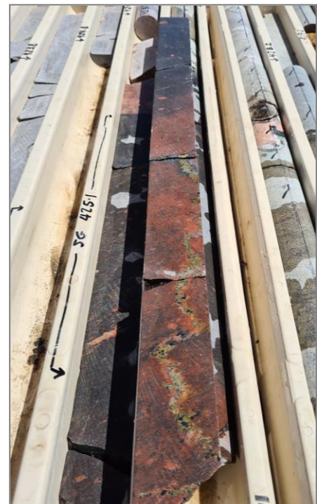
[Figure 12] Corkwood Project: Porphyritic volcanic rock showing early magnetite-biotite alteration (black colour at the top) demagnetised by red feldspar-silica alteration and associated chalcopyrite (weak magnetite) veining.
