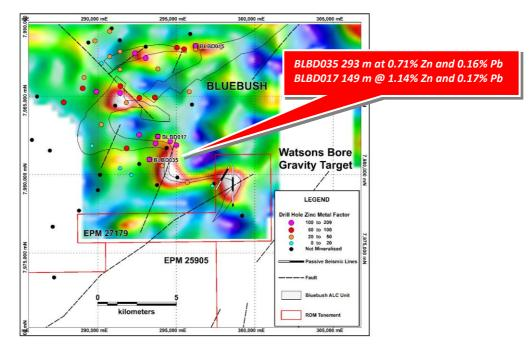
[Figure 5] Lawn Hill Project, Watson Bore tenement: Vertical gradient gravity imagery over the Bluebush area showing historic drill holes and thematic zinc metal factor (zinc weight % times intercept metres), the untested Watson Bore gravity target on Red Metal's EPM27179 and the recently completed passive seismic lines.
