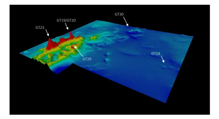
[Figure 8] Gidyea Project: 3D oblique topographic view facing northwest of the total magnetic intensity image (top). Key magnetic and gravity targets considered prospective for IOCG breccia deposits are labelled.
