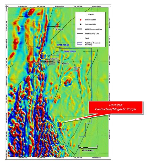
[Figure 10] Three Ways Project: Vertical gradient magnetic image showing moving loop ground electromagnetic lines, the 2020 drill holes TWD2001 and TWD2002 and the 2021 drill holes TWD2104, TWD2104 and TWD2105. Discrete magnetic targets adjacent to large structures are being considered for their copper potential.
