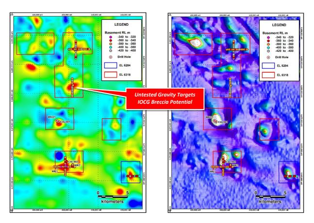
[Figure 14] Callabonna Joint Venture Project: Vertical gradient gravity image (left) and magnetic image (right) showing existing drill holes and the recent passive seismic lines with depth to basement estimates plotted thematically.
