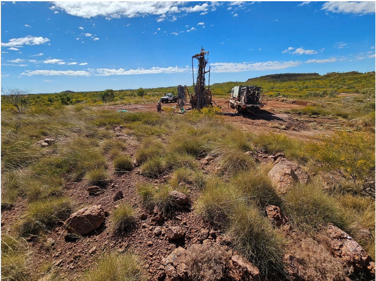
[Figure 1] Sybella Project: Percussion drilling with exposure of the REO enriched granite in the fore ground
