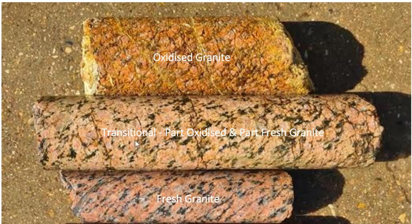
[Figure 1] Sybella Project: REO-enriched granite, oxidised, transitional and fresh. Note the coarse grain-size, weak biotite deformation fabric and increased fracture density with increased weathering.
