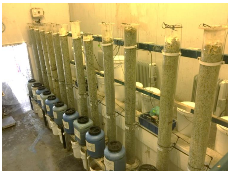
[Figure 2] Sybella Project: Intermittent bottle roll leach tests or IBRT (left), example of column leach tests (right).
