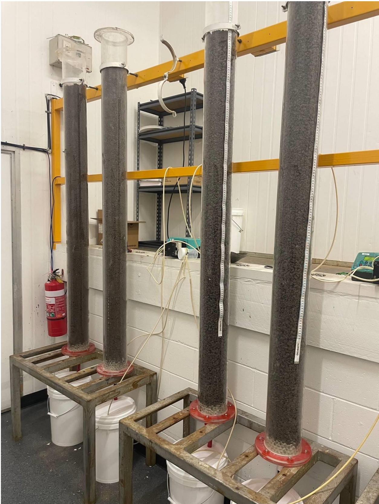
[Figure 5] Sybella Project Colum Leach Tests: Two metre, 150mm diameter columns filled with 15mm jaw crushed fresh granite being leached with weak sulphuric acid at pH 3 and pH 3.5 until terminal REO extraction over a residence time of about 120 days.
