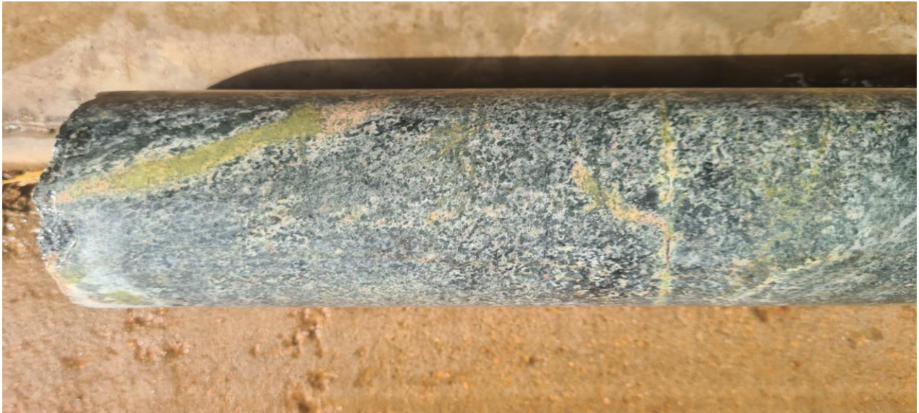
[Figure 5] Gulf 25GUD001: Typical weak altered gabbro with minor feldspar-epidote veins. Wide intercepts of this dense mafic rock type appear to explain the source to the gravity anomaly.
