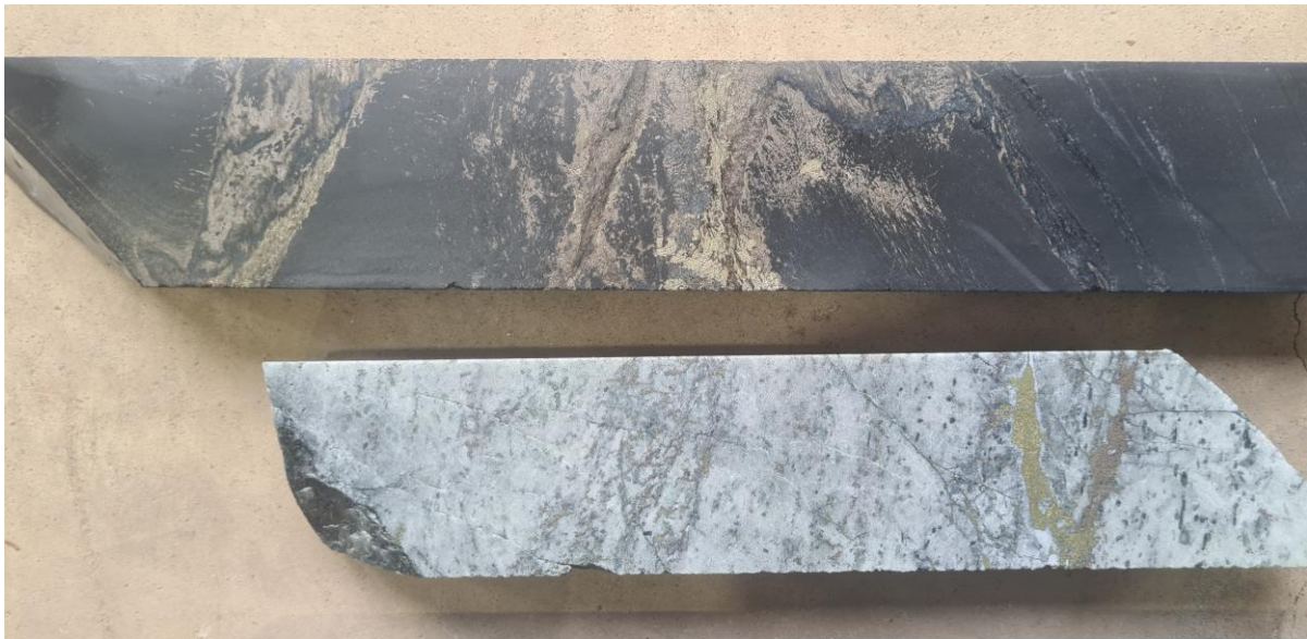
[Figure 1] Three Ways TWD25006A: Typical carbonaceous shale (top) and marble (bottom) with veins and disseminations of magnetic pyrrhotite some pyrite and minor chalcopyrite (copper sulphide). The iron sulphide bearing carbonaceous shale appears to have contributed to the source of the geophysical target. Assay results are pending.
