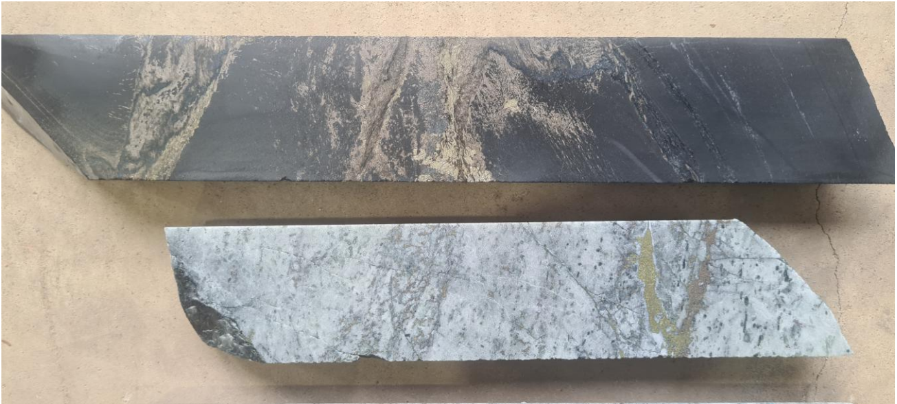
[Figure 9] Three Ways TWD25006A: Typical carbonaceous shale (top) and marble (bottom) with veins and disseminations of magnetic pyrrhotite some pyrite and minor chalcopyrite (copper sulphide). The iron sulphide bearing carbonaceous shale appears to have contributed to the source of the geophysical target. Assay results are pending.
