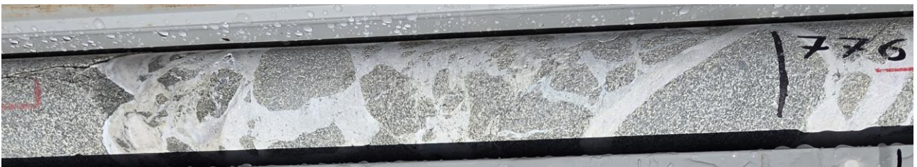
[Figure 5] Pulkarrimarra West: YE02, 25PWDD001B core photographs showing metasomatic replacement, spotting and veins of actinolite-feldspar-carbonate-biotite-quartz \pm pyrite rare pyrrhotite, strong wall rock biotite growth and blackening (top and middle), plus later-stage quartz-carbonate-sericite veinlets (top and middle) and quartz breccias (lower). Minor pyrite occurs along reactivated cleavage surfaces and in late-stage veins (middle).
