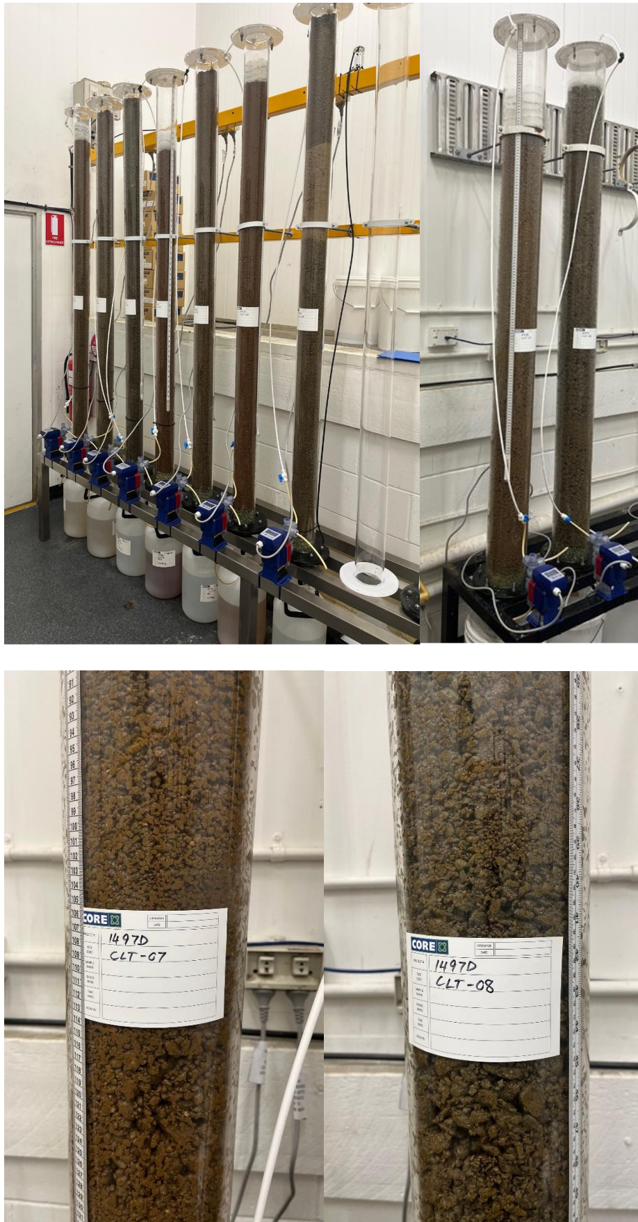
[Figure 11] Sybella Kary Zone: Column set-up showing 100mm and 150mm columns (top) and the crushed -20mm mineralisation in the columns (below).
