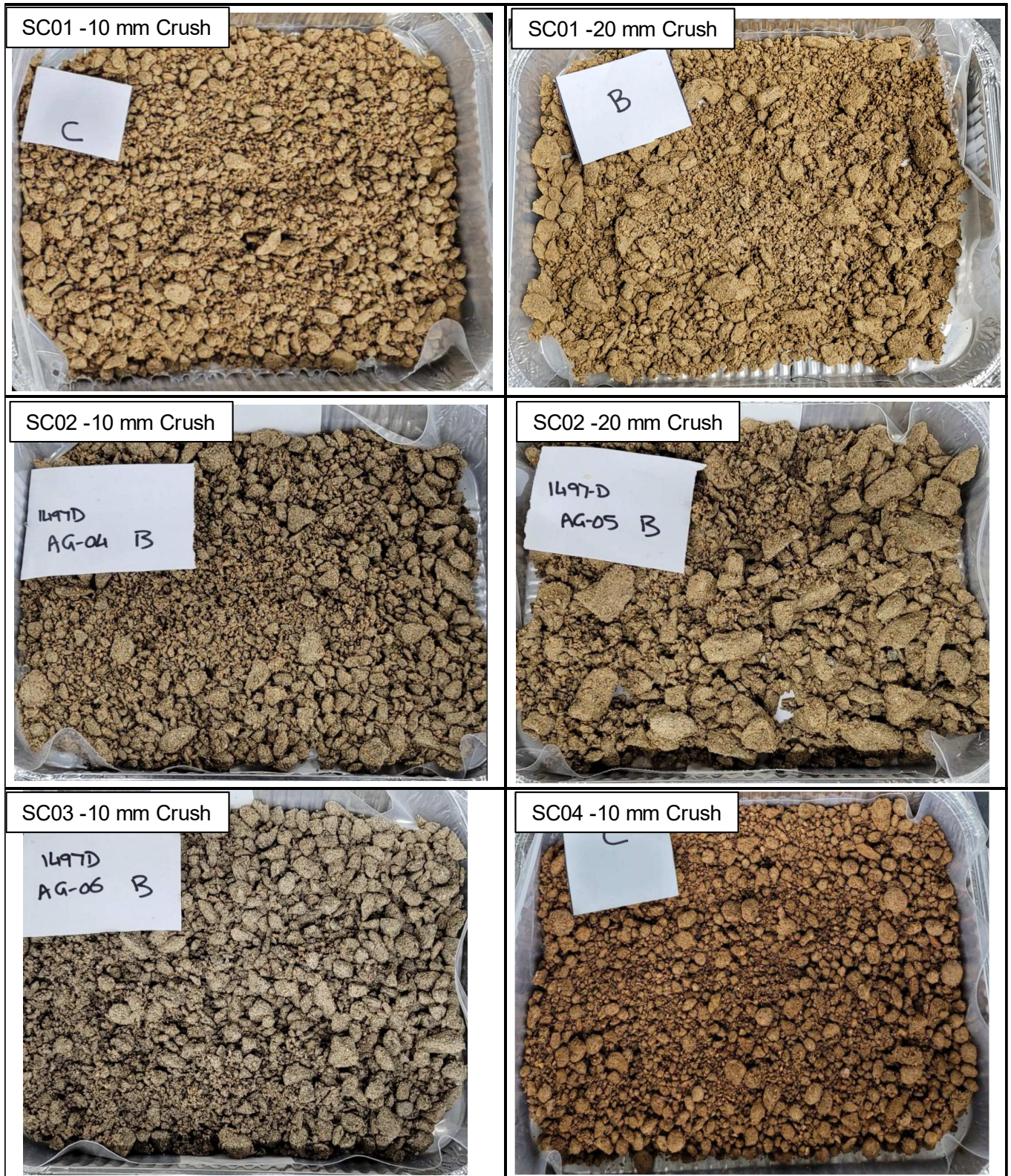
[Figure 10] Sybella Kary Zone: Acid agglomerated crushed mineralisation prior to being placed in the column.
