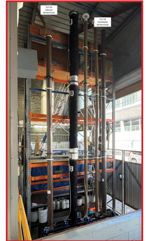
6m columns leach testing in progress
